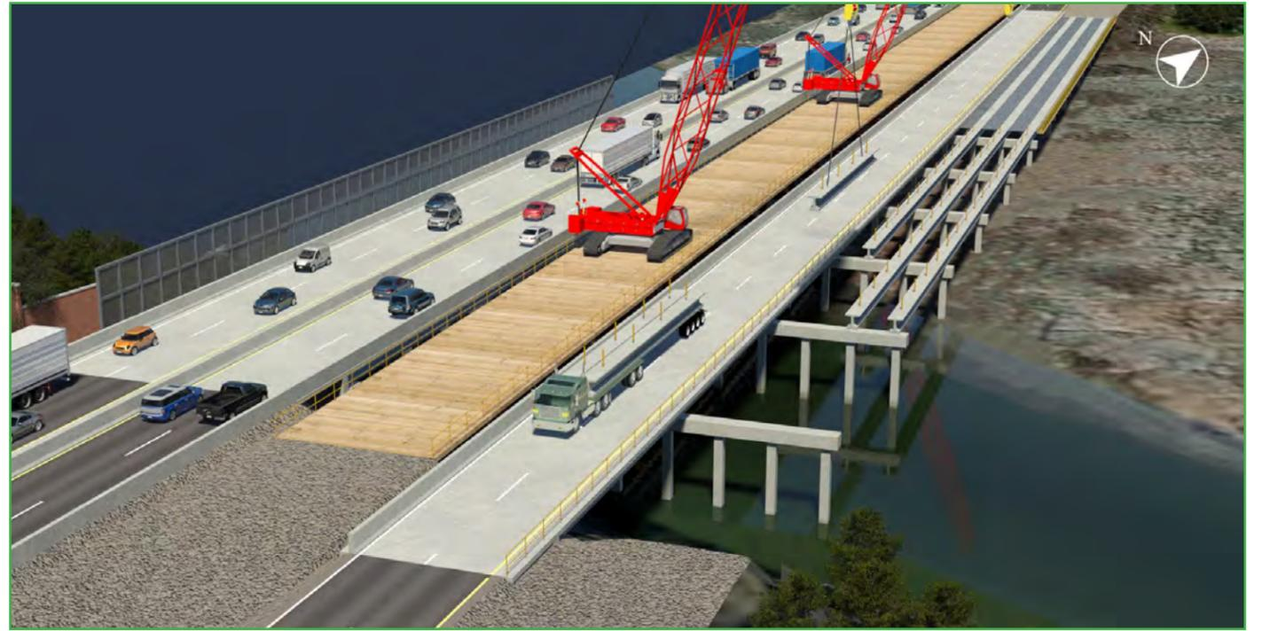
Figure 4.7.16: Install superstructure.
