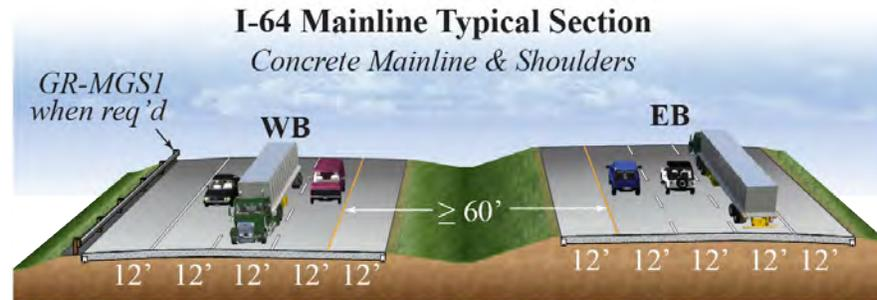
**Figure 4.3.2: Concrete Mainline and Shoulders.** This typical section offers durability and functionality, with readily available source materials.
