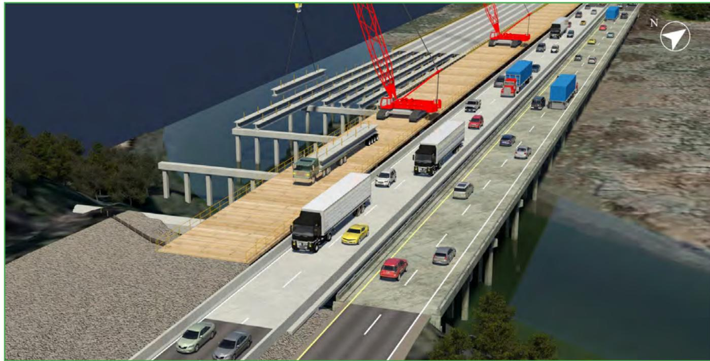
Figure 4.7.11: Install superstructure.
