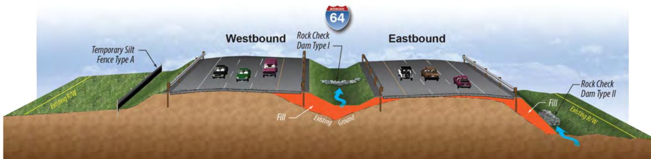
**Figure 4.4.8: Reconstructing of Slope.** The Skanska Team will use slope stability checks to ensure that the roadway, work zone, and utilities are safe and secured.
